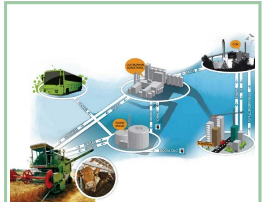
By means of industrial symbiosis, sustainable biofuels for transport is produced showing a world class GHG performance. Industrial symbiosis is a cooperation to find synergies in order to produce a joint result that is better than the sum of the individual parts. In the case of bioethanol from grains, a GHG reduction of more than 90% is achieved compared to gasoline and diesel.
